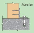
For a soft surface, timber stakes should be driven into the ground and the legs of the arbour fixed to them.
