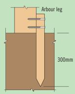
Arches have longer legs and should be embedded into soft ground. Fix the legs in place using a post-fix product such as MetCrete.
