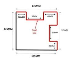
Concrete Corner Post 2.48m x 135mm thick by 125mm wide. - Approx slot length 74 inch (1880mm) for fence -For a 6ft (1.8m) overall height finish. - Steel reinforced concrete corner post - Slotted 2 sides - No minimum order quantity for Del Area A - Not available for delivery in Del Area B
