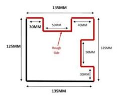
Concrete Corner Post 1560mm x 135mm x 125mm - Steel reinforced concrete corner post - Slotted 2 sides -Weight per post: 48.7kg - No minimum order quantity for Del Area A - Not available for delivery in Del Area B CHECK MY DELIVERY AREA
