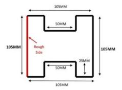
Concrete inter post 1.58m high x 105mm thick by 105mm wide.
