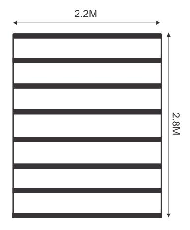
We reserve the right to alter design without prior notice. If it is crucial that the floor joists run the same direction as shown above, this must be stated on the order.
