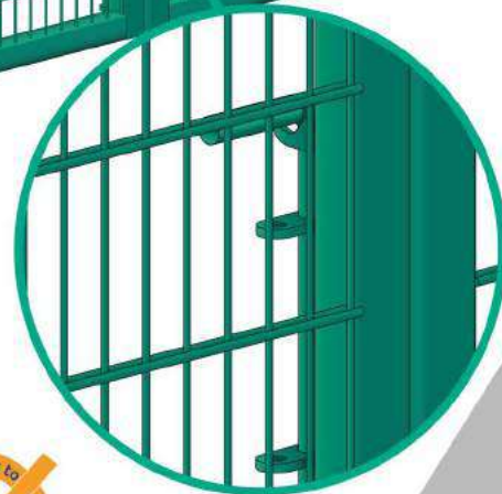
Padlockable Drop Bolt Detail
