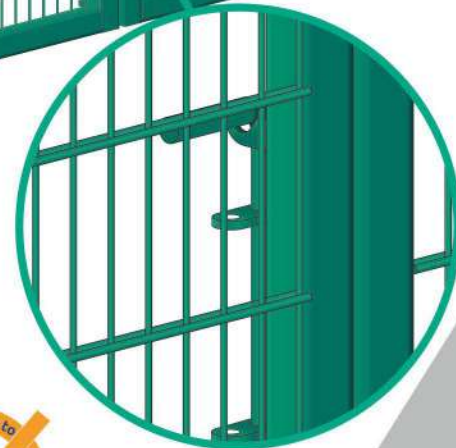
Padlockable Drop Bolt Detail
