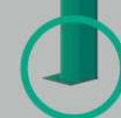
Ragging plates to key into concrete foundation
