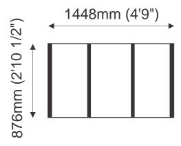
If using bearers we suggest 2 at 5ft (1.5m) We reserve the right to alter design without prior notice. If it is crucial that the floor joists run the same direction as shown above, this must be stated on the order.
