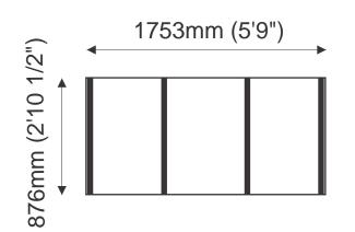
If using bearers we suggest 2 at 6ft (1.8m) We reserve the right to alter design without prior notice. If it is crucial that the floor joists run the same direction as shown above, this must be stated on the order.
