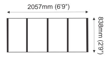
If using bearers we suggest 2 at 7ft (2.1m) We reserve the right to alter design without prior notice. If it is crucial that the floor joists run the same direction as shown above, this must be stated on the order.
